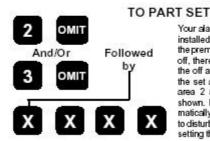
Your alarm system may have been installed to allow you to to have part of the premises set while other area(s) are off, thereby allowing free access with the off area(s), and alarm protection in the set areas. To set the system with area 2 and/or 3 omitted, proceed as shown. Note that the exit tone is automatically reduced by one third so as not to disturb sleeping occupants when part setting the system.
